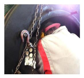
**Steam loco B10**'s front tube plate continues to receive attention prior to refitting her boiler tubes. A pressure vessel certified welder has repaired four small imperfections in the plate surface. These welds have since been machined flat and the four adjacent holes re-machined to ensure a snug fit for the tubes. It is hoped that the loco will be running again before the summer season.
